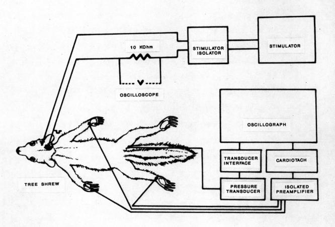
Fig.1. Diagrammatic picture of experimental arrangements routinely employed in experiments involving electrophysiological invertigation
