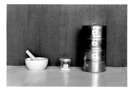
Fig. 4.1 Unit for grinding and Screening Support
