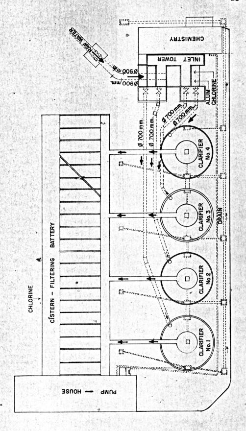
Fig. 3.3 The Flow Diagram of Thonburi Water Treatment Plant.
