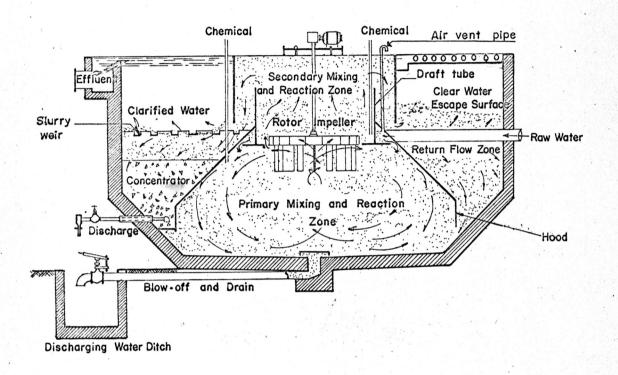
The Accelator consists essentially of a basin in which is contained:
