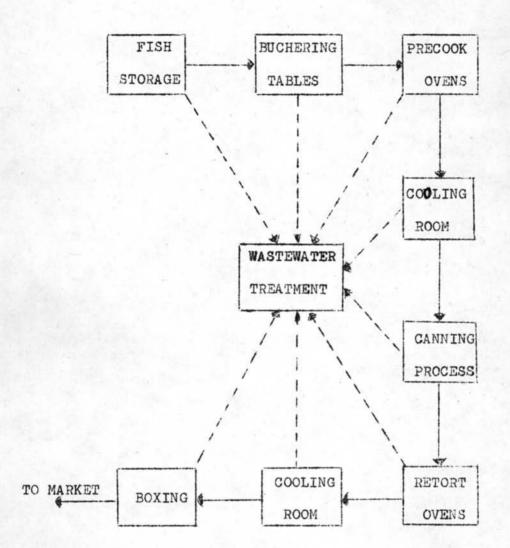
Figure 2.1 FISH CANNING PROCESS AND WASTEWATER GENERATION.
