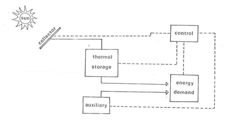
Figure 1 The overall solar-thermal system. Solid lines represent energy flows; the dash lines information flows
