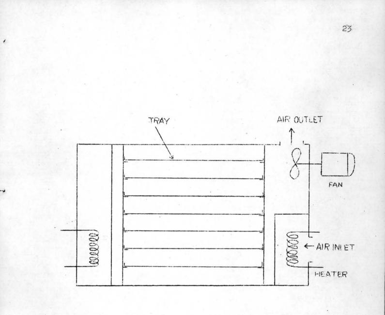
Fig. 3 Compartment Tray Dryer
