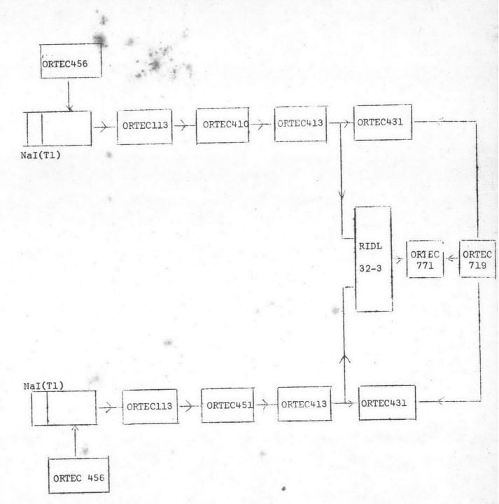
Fig. 4 Block diagram of the coincidence counting system arranged for the experiment.
