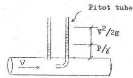
The difference in elevation  $\sqrt[-v^2/2g]$  of fluid in the two tubes  $\frac{P}{\delta}$  represents the velocity head,  $v^2/2g$  (Vennard, 1961) In opposite case, if it is faced downstream, the elevation of fluid in the Pitot tube will drop down causing lower level than that of the straight tube, thus gains the velocity head as an additional suction unit if the loss due to the Pitot tube is negligible. The equation concerned will be:-
