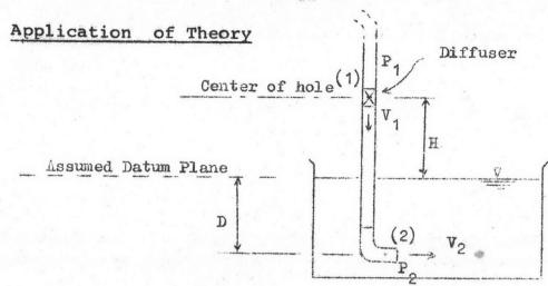
When all holes of the diffuser are closed, the engergy equation between Section (1) and Section (2) of the pipe shown in the above figure is as following:
