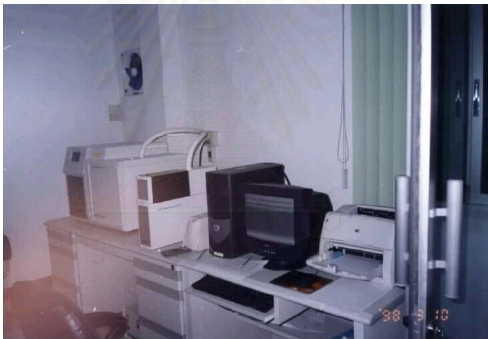
Figure 3.3: Analytical equipment; GC/FID- Varian CP-3800, with 0.32 mm ID x 60-m length-CP-Sil5 CB-capillary column
