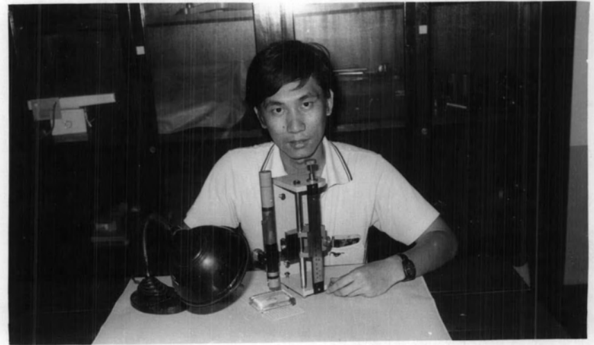
Fig.4-10. The use of the constructed traveling microscope in vertical position.
