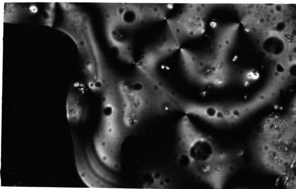
Fig.9b Inversion walls of the second kind joining the +\frac{1}{2} and -\frac{1}{2} point singularities of MBBA(dirty) at 41.35^{\circ}\text{C} . Crossed polarizers.
