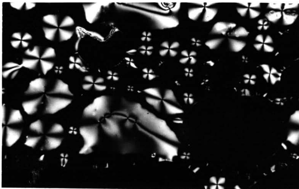
Fig.13a Partially pseudo-isotropic texture of PAA/EPP-Hep 50% at 114.3^{\circ}\text{C} . Crossed polarizers.
