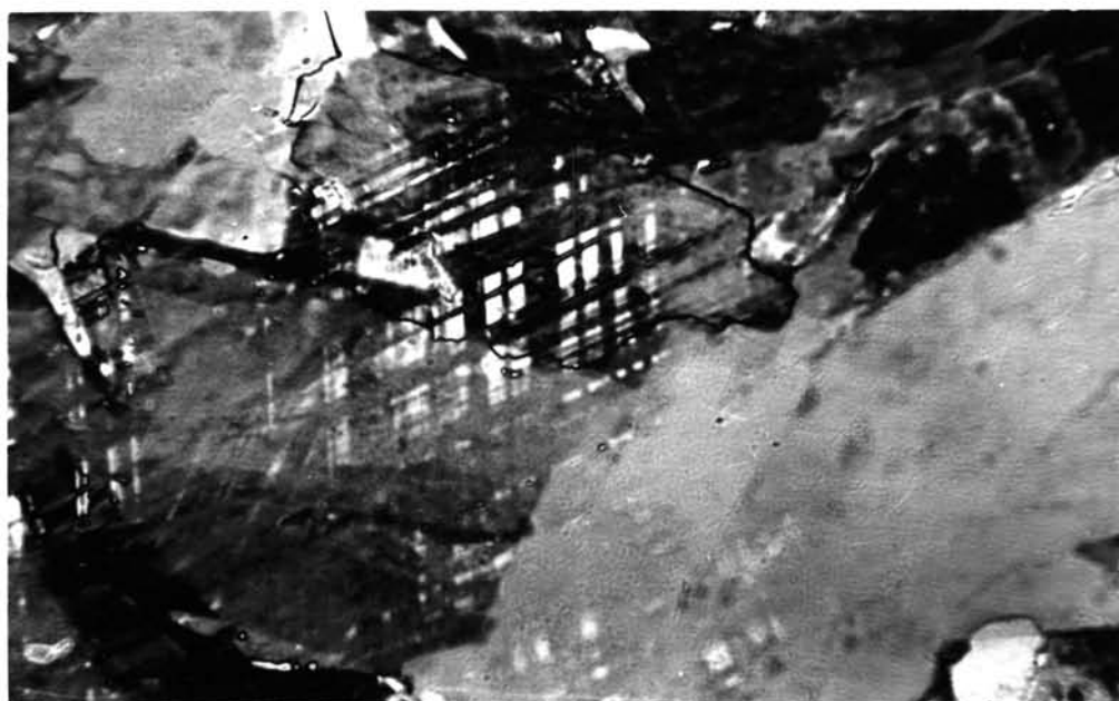
Fig.7a Marbled texture of EPPV at 122.6^{\circ}\text{C} . Crossed polarizers.
