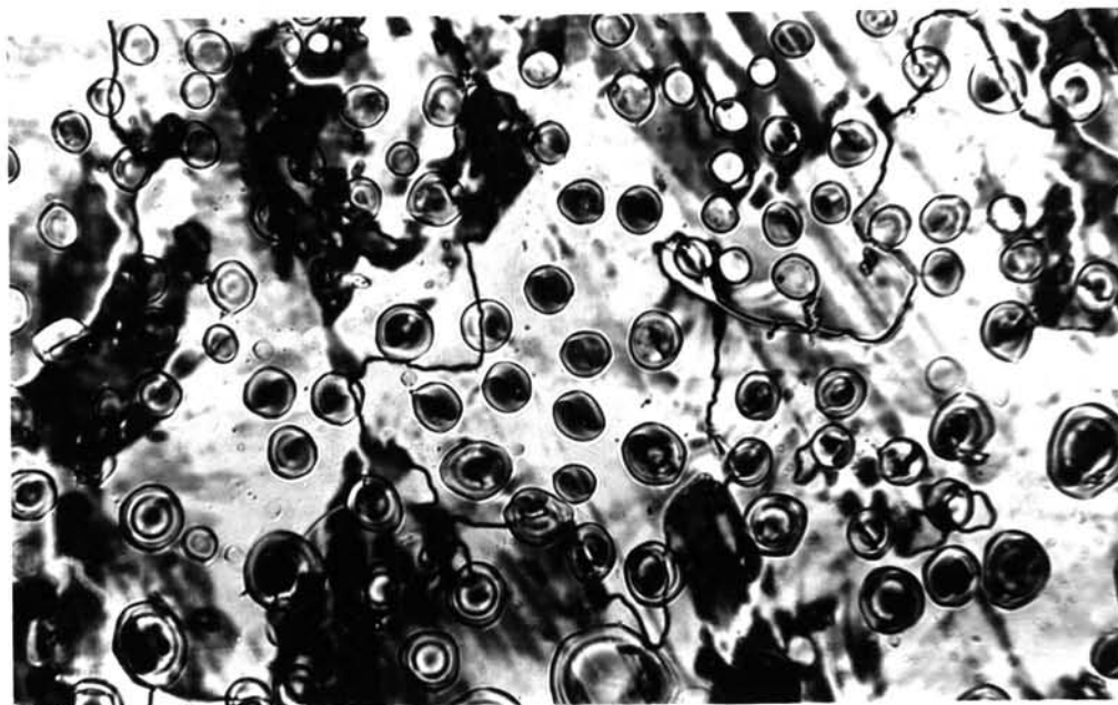
Fig.6b Texture of EPP-Hex (recryst.) at the nematic-isotropic transition at 128.4^{\circ}\text{C} , under crossed polarizers.
