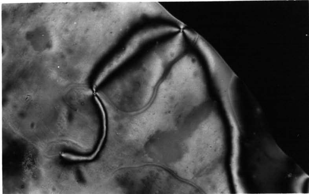
Fig.8b Schlieren texture of PDBAB at 135.6^{\circ}\text{C} exhibited by the same sample as that shown in Fig.8a.
