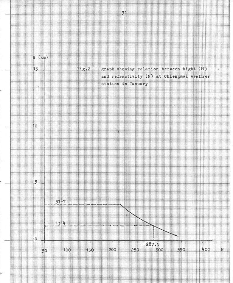
From graph the value of N at elevation of 1314 metres above mean sea level or at the height of 1 kilometre above the earth's surface is 287.5
