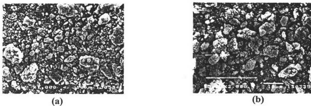
Figure H11 SEM photographs: Pth_200:1/MOR_40 at magnification (a) 1000 and (b) 2000.
