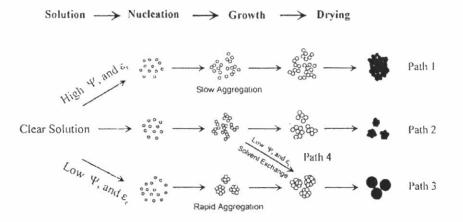
Figure 2.1 Schematics of particle growth in the mixed solvent of alcohol and water. (Park *et al.*, 1997)
