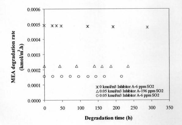
Figure 6.3 Degradation rate-time plots of MEA-O<sub>2</sub>-SO<sub>2</sub>-H<sub>2</sub>O system with 0.05 kmol/m<sup>3</sup> Inhibitor UR-A (5 kmol/m<sup>3</sup> MEA, 6% O<sub>2</sub>, 393 K).
