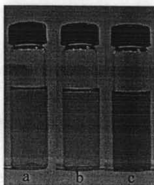
Figure 4.22 Photograph of synthesized silver nanoparticles by various synthesis methods: (a) thermal reduction of sprayed silver salt, (b) precursor injection, and (c) precursor heating method.
