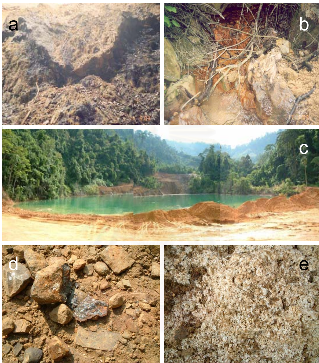
Figure 4.1 Anthropogenic sources of metals at the Euro-Thai abandoned mine. (a.) A waste pile dumped at the bank of the stream. (Long-axis of photograph is about 1.5 m.) (b) Reddish drainage from the waste pile. (c) The artificial pit (about 70 x 100 x 60 m 3 ) with strongly contaminated greenish-colored water. (d) Dumped waste rocks for road access to mine site. (e) Strongly weathered disposed wastes near the mine site.
