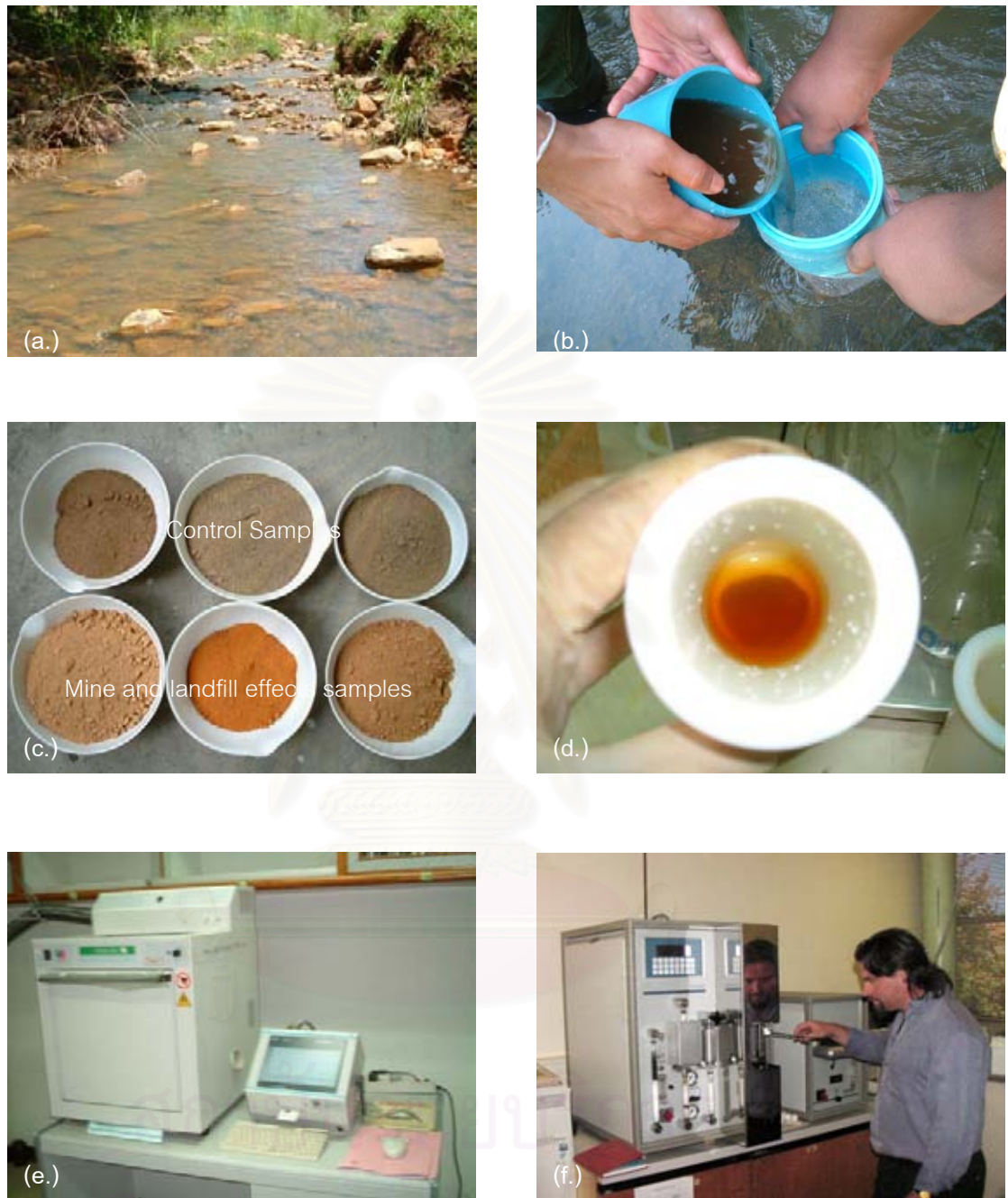
Figure 3.2 (a.) The main stream at location 740988E 0692067N in the study area, (b.) Wet sieving using stream water in the field, (c.) Dried samples before being dry sieved, (d.) Filtration after adding mixed acid, (e.) Microwave model digester and (f.) Eltra CS 4000 Carbon and sulfur determinator.
