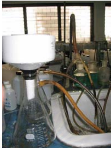
Buchner funnel for extracting leachate (solution).
