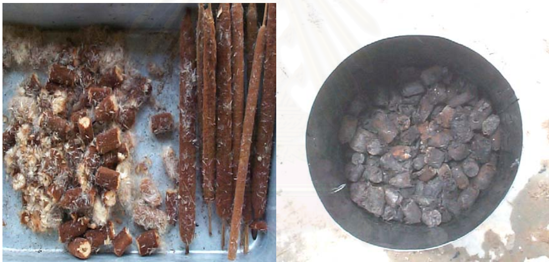
Figure C.3 Cattail fiber: Before and after
