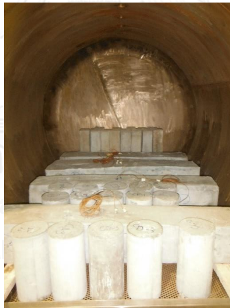
Figure 0-7 RPC in autoclave
