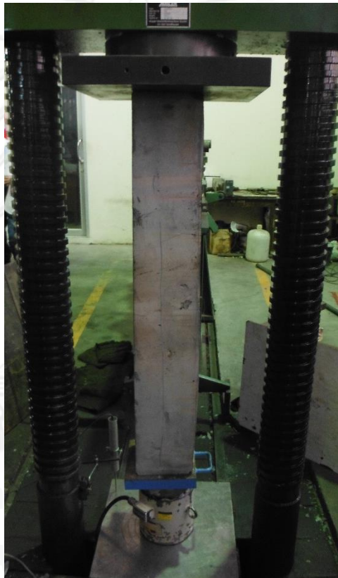
Figure 0-11 Test setup of Specimen COL-A
