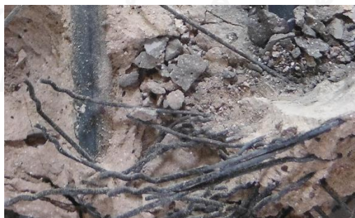
Figure 0-15 COL-C: Color change and bending of fibers
