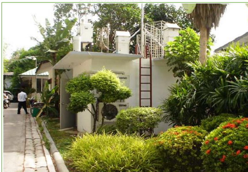
Figure 3.3 Air pollutants sampling points over PCD Air Quality Monitoring Station at Bansomdej Chaopraya Rajabhat University Station
