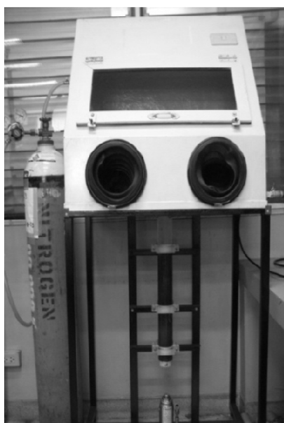
Figure 3-4 Nitrogen glove box for handling sediment samples under oxygen-free (nitrogen) atmosphere
