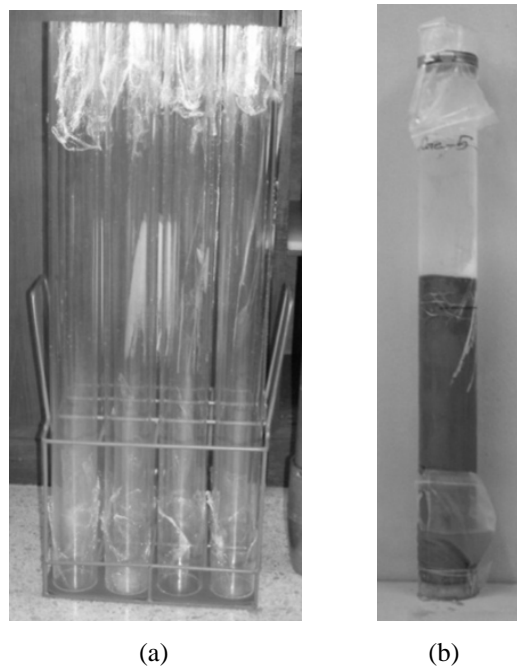
Figure 3-3 Push corers (a) Push corers making from Plexiglas ® , and (b) Plexiglas containing sediment
