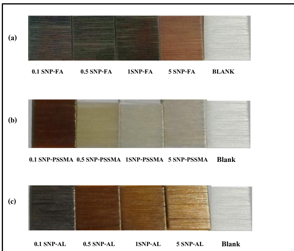
Figure 4.24 PEM of PDADMAC and SNP coated on polyamide suture material. (a) PDADMAC/SNP-FA 20 layers, (b) PDADMAC/SNP-PSSMA 20 layers and (c) PDADMAC/SNP-AL 20 layers.
