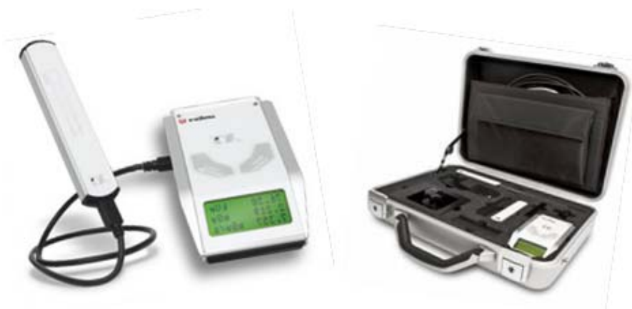
Figure 3.2 Solid state detector systems, Unfors model XI [10, 11].
