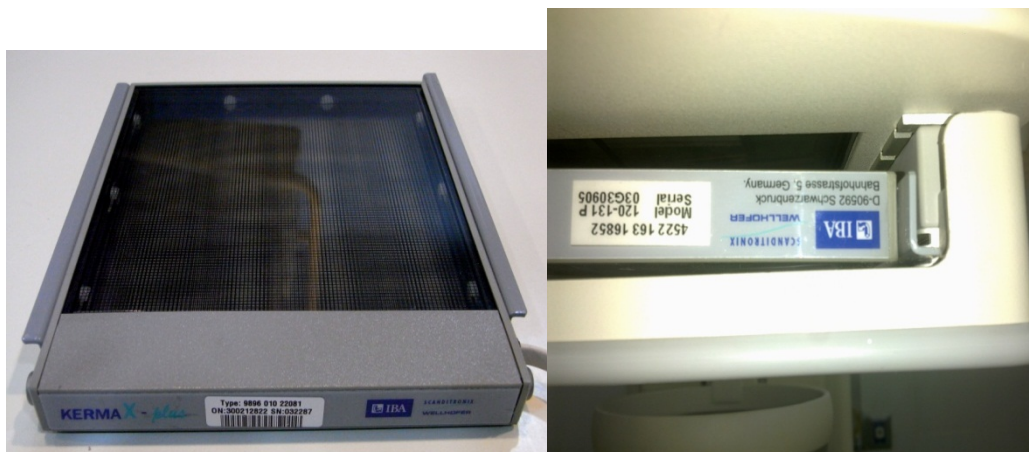
Figure 3.3 DAP meter placed on an x ray tube with the readout value on display monitor.
