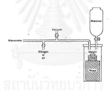
Figure 2.6 The apparatus of impregnation process [14]
