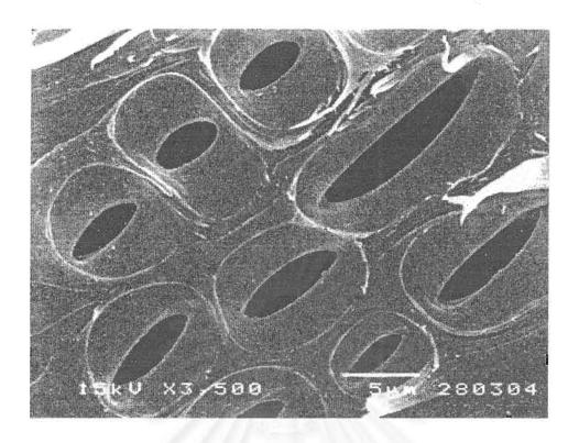
Figure 4.11 SEM micrograph of transverse section of empty wood cells (3,500 x)
