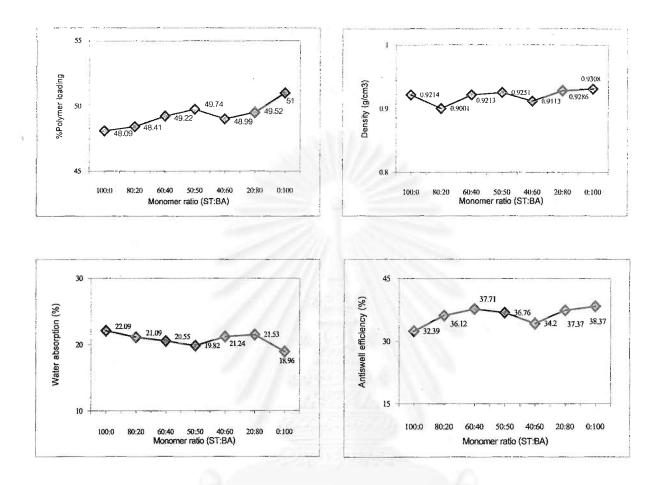
Figure 4.7 Effect of monomer ratio on physical properties prepared from various monomer ratios (ST : BA)
