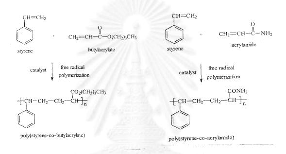
Figure 2.5 Preparation of poly(styrene-co-butylacrylate) and
