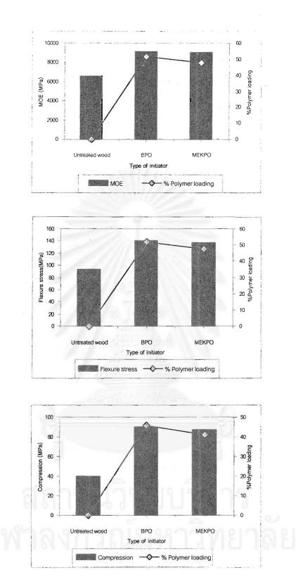
Figure 4.4 Comparison of mechanical properties of WPC samples treated with BPO and MEKPO and natural para rubberwood
