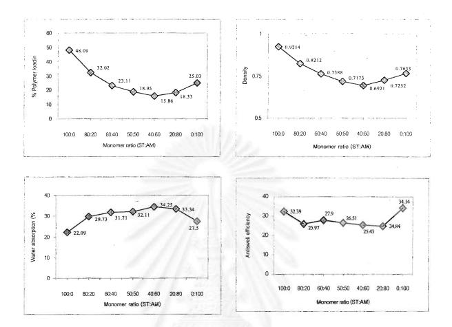
Figure 4.9 Effect of monomer ratio on physical properties prepared from various
