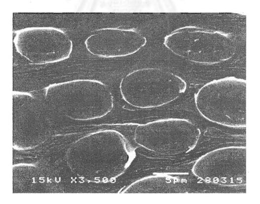
Figure 4.12 SEM micrograph of transverse section of polymer filled cells (3,500x)
