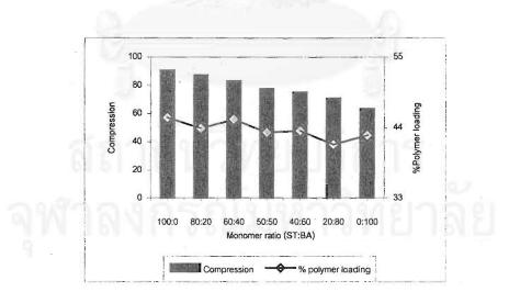
Figure 4.8 Effect of monomer ratio on mechanical properties prepared from various monomer ratios (ST : BA)
