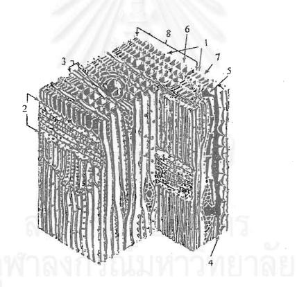
Figure 2.3 Magnified three- dimensional diagrammatic sketch of softwood:
