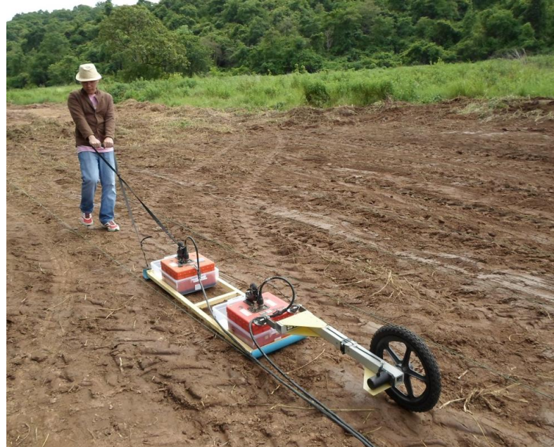
Figure 3.6 GPR with FO method was towed along survey line for data collecting.
