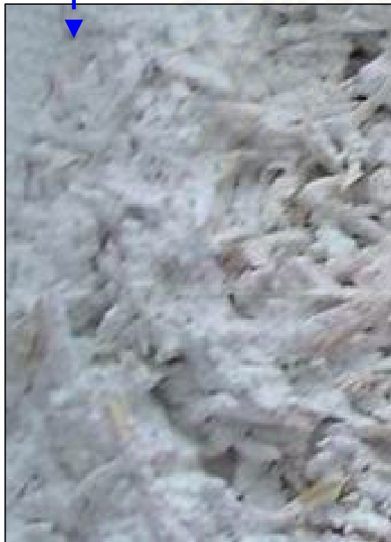
Figure 4.17 (b) A zoomed-up photo of dust cake layer was revealed. Obviously, the layer was a nonuniform patchy combination of calcium carbonate dust and rice husk particles.
