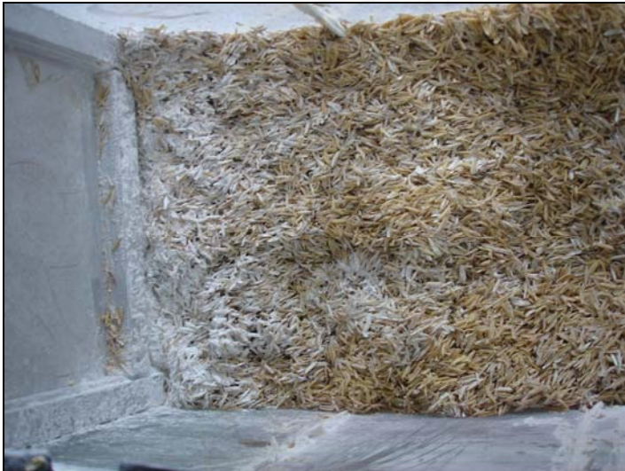
Figure 4.19 Front view of the filtration area showing the formation of patchy dust cake layer (The net screen is clearly visible) [Taken after 2 hours of operation, at 0.81 m/s of face velocity, and 0.5 m. of media thickness]
