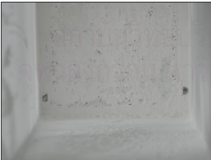
Figure 4.20 Another front view of the inlet filtration area showing the formation of non-uniform dust cake layer (The net screen is clearly visible) [Taken after 2 hours of operation, at 0.63 m/s of face velocity, and 0.125 m. of media thickness]
