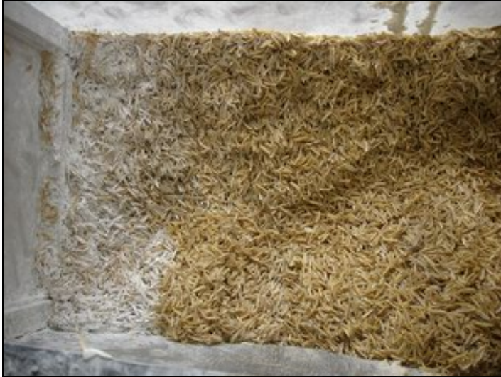
Figure 4.18 Another photo illustrating the formation of dust cake layer as well as dust penetration. [Taken after 2 hours of operation, at 0.63 m/s of face velocity, and 0.5 m. of media thickness]
