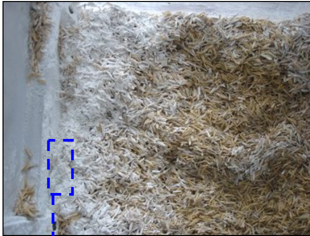
Figure 4.17 (a) Dust particles deposited, accumulated, and formed a non-uniform patchy dust cake layer while penetrating and partially passing through the bed [A photo taken after 2 hours of operation, at 0.63 m/s of face velocity, when thickness of media filter was 0.25 m.]
