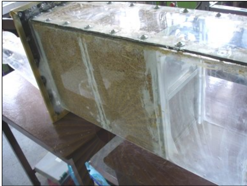
Figure 4.15 Well packed rice husk media filter in the media box.
