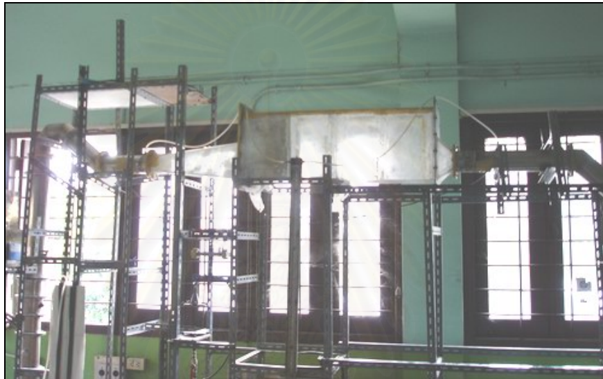
Figure 4.3 A photo of the side view of the laboratory-scale unit. The media box, lies on left side of the rectangular box, in the center.
