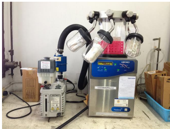
Figure 9 Freeze-dried lyophilization used to increase the concentration of produced biosurfactant
