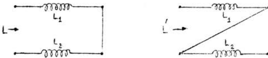
Fig.3-14 Equivalent circuit of H.V. and L.V. coil for measurement of Mutual inductance.
