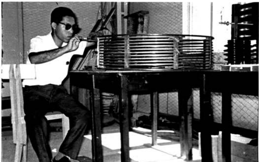
Fig.2-9 Winding of the Low Voltage coil.
