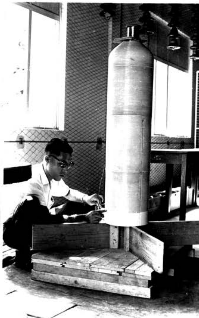
Fig.2-2 Winding of the High Voltage coil.
