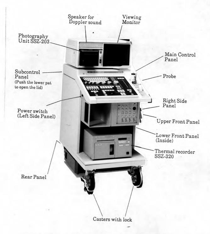
Fig.2 Echocardiographic machine ( Aloka Color Doppler model SSD-870 )
