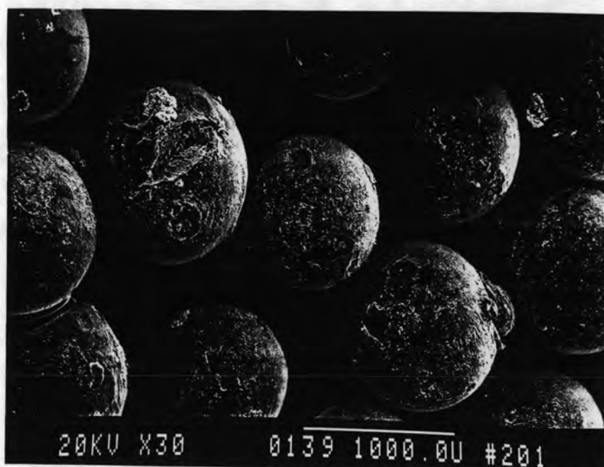
Figure 31 SEM micrograph of the surface of the large beads (S-T2/N3) Diluent: toluene
