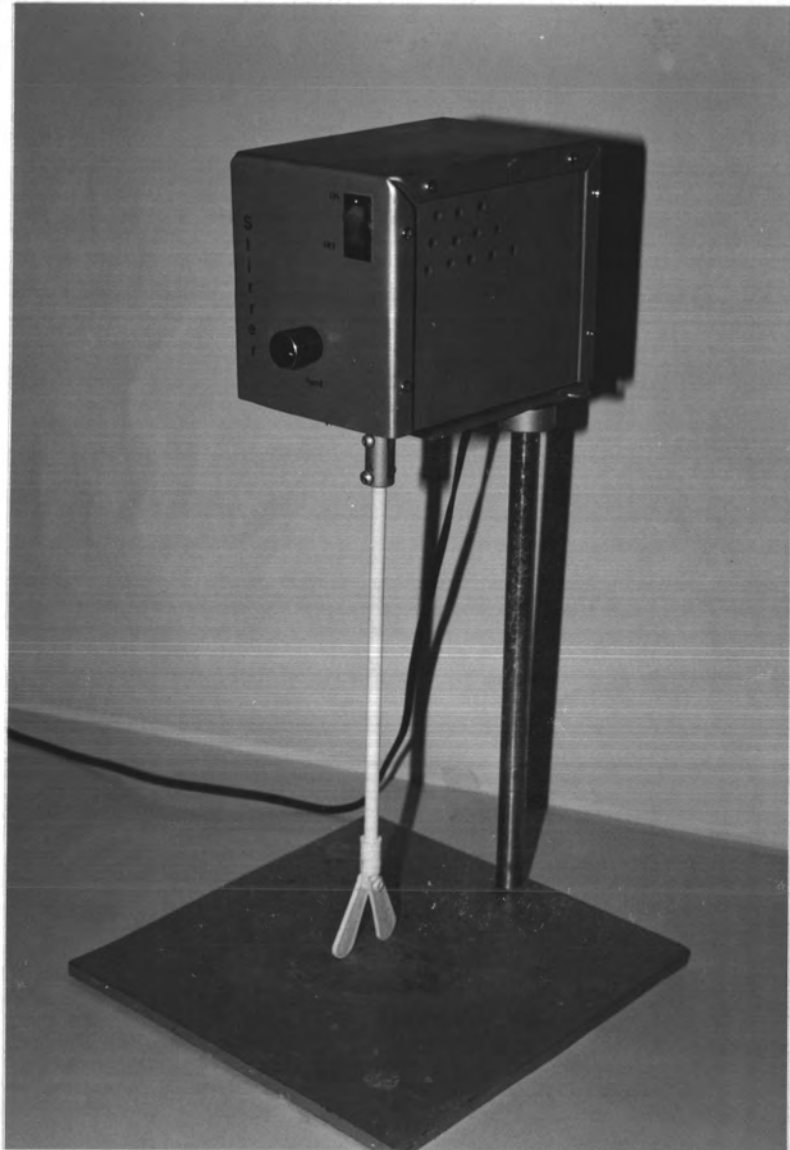
Fig.2.1 Photograph of adjustable speed stirrer with teflon paddle.
