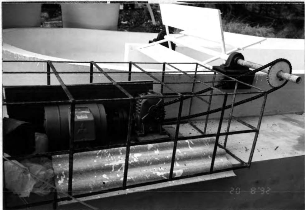
Figure 41. Four blade paddle wheel driven by motor and reducing gear for the water circulation.
