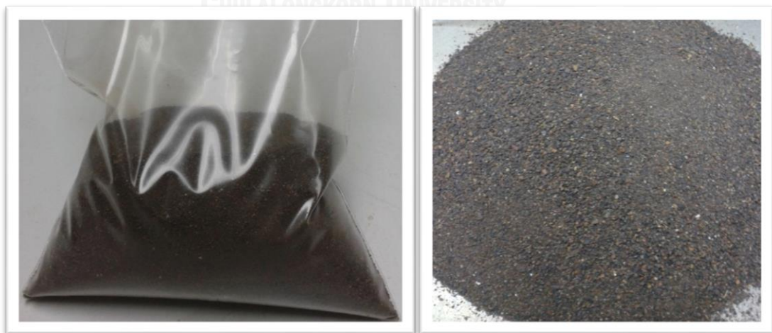
Figure 3. 1 Tin concentrate samples from shaking tables of Lao-Korea mining company, Khammouane Province, Lao PDR
