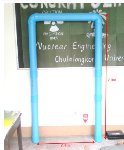
Figure 3.8 The PVC portal gate in the walk-through RMS.
