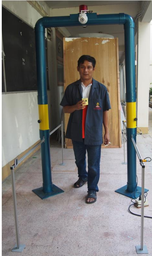
Figure 4.10 The person brings the radioactive source (contained in yellow box) to test the system.
