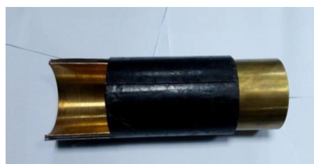
(b) Lead Shielding of the detector
