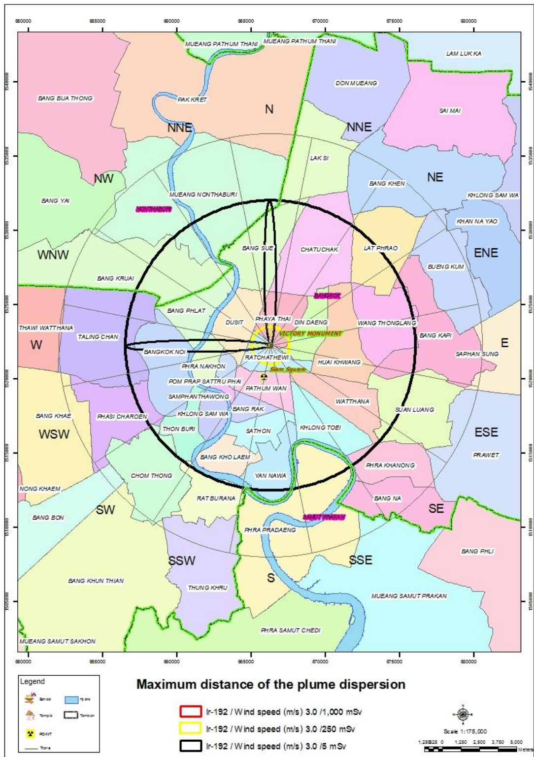
Figure 4.14 Boundary of affected areas at the Victory Monument site for the case of Ir-192 with high explosive of 25 pounds and wind speed of 3.0 m/s blowing from S and E directions
