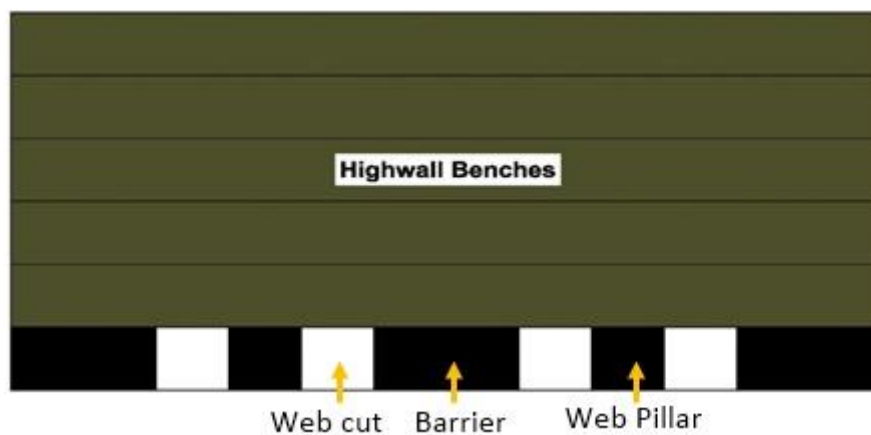
Figure 2-4: Continuous highwall mining geometry.
