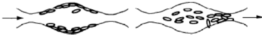
Figure 2.1 Reduction of salinity in injected brine causes release of clays from pore walls, resulting in blocking of pore throat entry, a process is so-called log-jamming [8]
