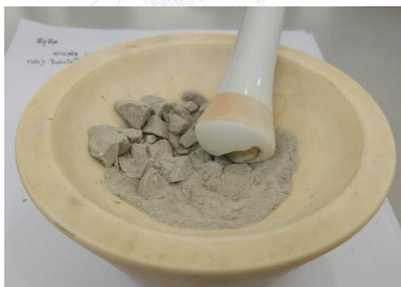
Figure 4.1 Grinded rock sample by the use of ceramic mortar and pestle
