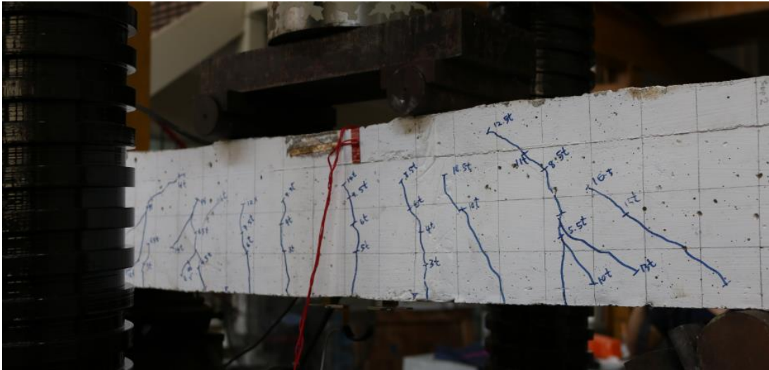
(c) Four point flexural beam test
