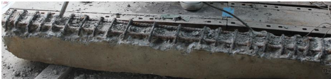
Figure 3.10 Breaking tension zone
