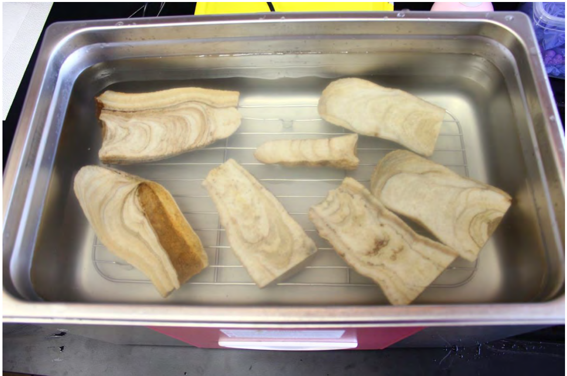
Figure 18. Washing sample in Ultrasonic cleaner machine with Deionized water.
