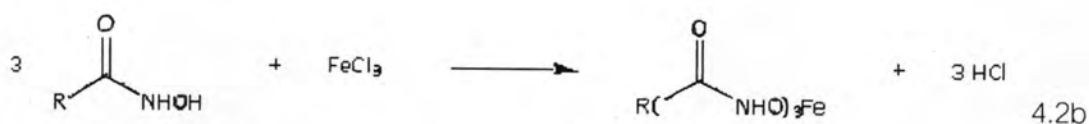
Figure 2.8 Colorimetry reaction of hydrolyzed AHL. 4.9a ; reaction of straight chain ester with hydroxylamine resulting in hydroxamic acid formation. 4.9b; the colorimetry reaction of hydroxamic acid with ferric chloride . The colored chelate complex product can be determined by spectrophotometer.
