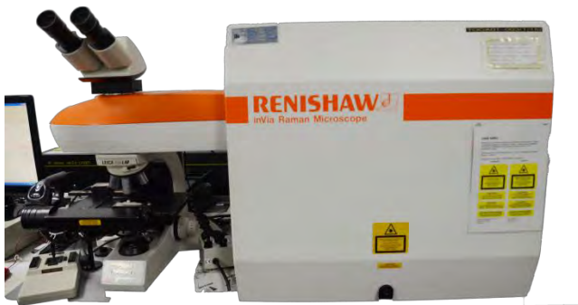
Figure 3.6 Laser Raman Spectrometer model Renishaw T00A01-003 based at the Gem and Jewelry Institute of Thailand (GIT)
