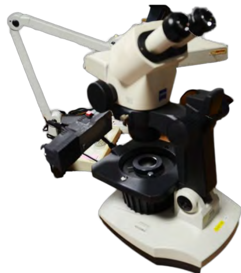
Figure 3.5 Gemological Microscope based at the Gem and Jewelry Institute of Thailand (GIT)
