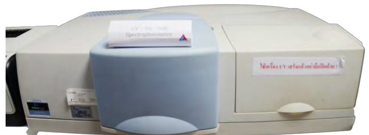
Figure 3.9 Ultra Violet-Visible Light-Near Infrared Spectrometer (UV-Vis-NIR) model Lambda 950 Perkin Elmer based at the Gem and Jewelry Institute of Thailand (GIT)
