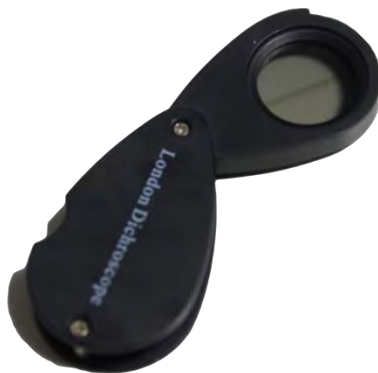
Figure 3.4 London Dichroscope based at the Gem and Jewelry Institute of Thailand (GIT)
