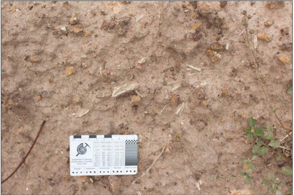
Figure 4-4 Pale brownish to brownish silt to clay sediments with laterite grains and quartz grains at the field observation station 7 in Figure 3-27
