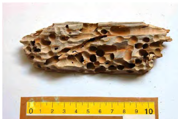
รูปที่ 20 Piece of driftwood heavily drilled by teredinid wood-boring bivalves. Note that the openings of borings are perpendicular to the surface, flattening at depth, being parallel to the wood grain. Scale in centimetres. Socotra, Yemen. (KÁZMÉR and TABOROŠI ,2012)
