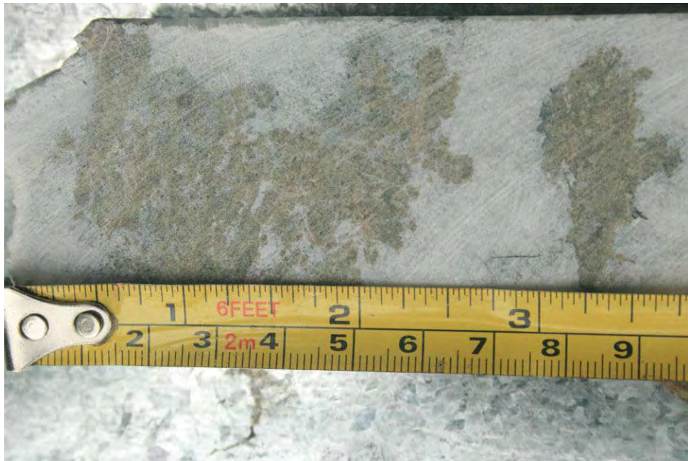
Figure 3-8: A slabbed core sample of marble showing coarse-grained, light grey calcite with large patches of garnet skarn replacement.
