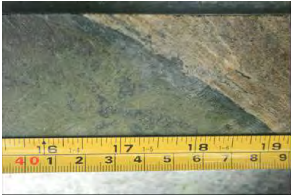
Figure 3-18: A slabbed core sample of reddish brown garnet skarn crosscut by epidote vein?
