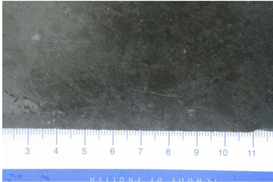
Figure 3-32: A slabbed core sample of andesitic lapilli tuff showing dark green to black, fine-grained rock and containing fragments varying from 0.1-3 cm.
