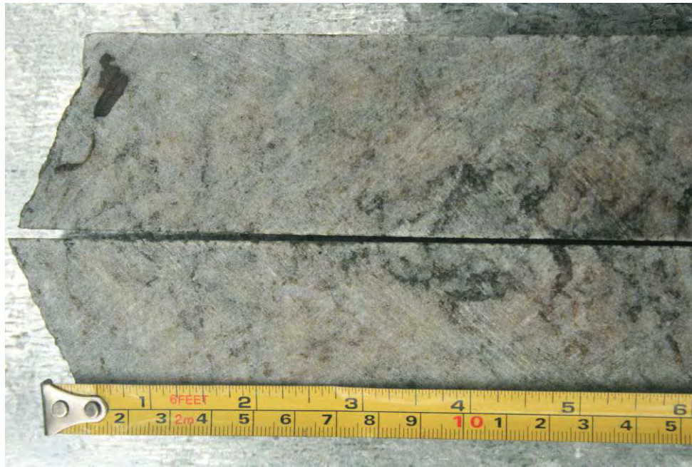
Figure 3-6: A slabbed core sample of marble showing fine to medium-grained calcite with patches of dark minerals.
