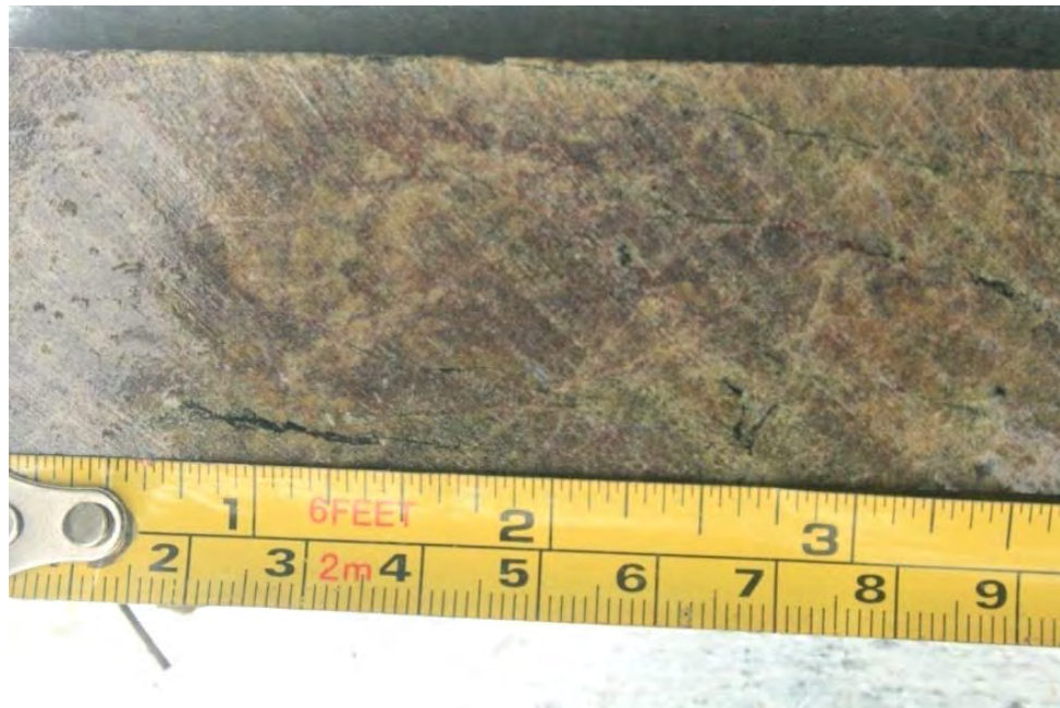
Figure 3-22: A slab core sample of garnet skarn showing coarse-grained garnet.
