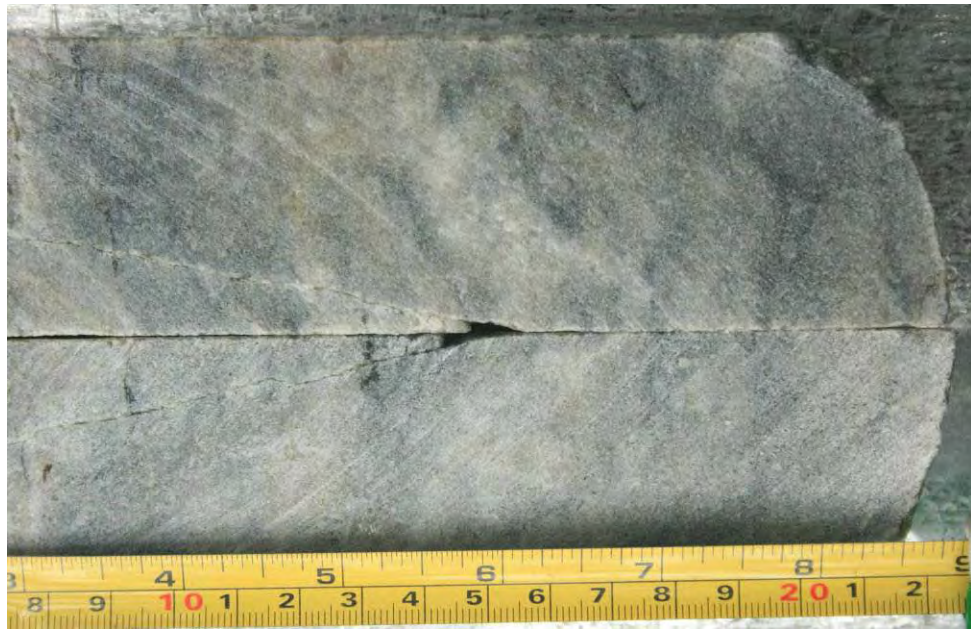
Figure 3-4: A slabbed core sample of light grey marble containing fine-grained calcite and patches of dark minerals.
