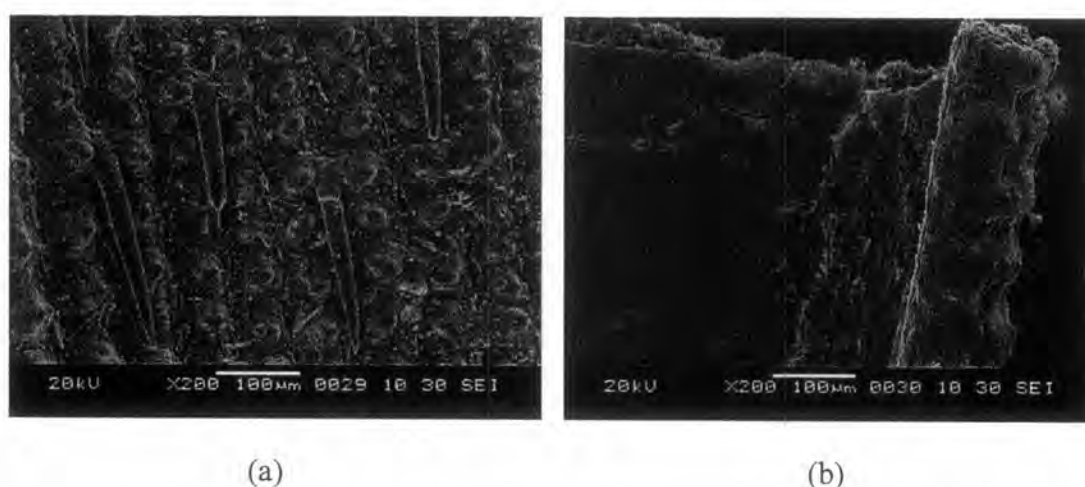
Fig. 2.4 SEM micrographs of outer epidermis (a) and inner epidermis of rice husk (b).
