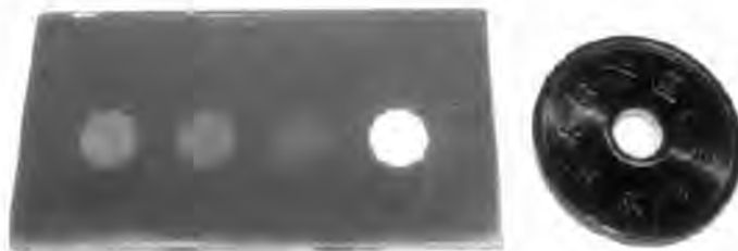
Fig. 2.26 A thick multicolored \text{Ag-TiO}_2 film. Each spot (6 mm diameter) was irradiated successively with a blue, green, red, or white light.
