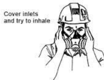
Negative- pressure test
